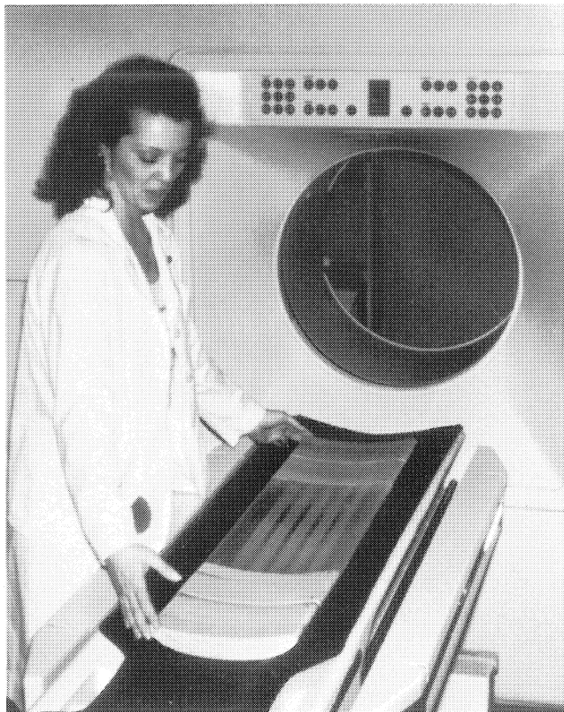
Figure 4. The mineral calibration phantom has five tubes embedded within it. The tubes contain standardized solutions of K_2HPO_4 , water, and a fat-equivalent solution of ethanol. To fit under the patient it is designed in the shape of a crescent.
