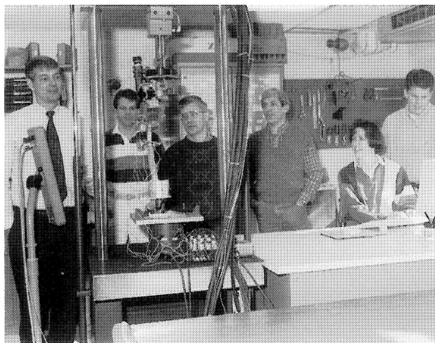
Figure 3 Discussing MTS set-up for torsional micro-motion testing of a new cementless femoral component design. Left to right: Dr. Tom Brown; Doug Adams (graduate student); Doug Pedersen (staff engineer); Jim Rudert; Erika Skaro; Dan Fitzpatrick (graduate students).
