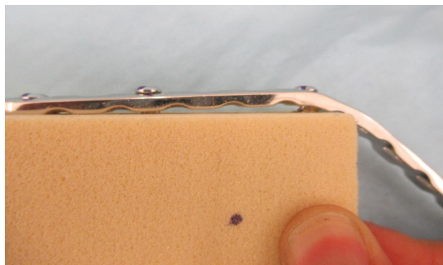
Figure 4. Close inspection of the failed 12-hole perpendicular, non-locked plates revealed that the plate bent at the rigid fulcrum such that an arc extended over the bone block. Compared to the gross bending of the plate concentrated at the fulcrum, this more subtle arc lifted the plate off the bone block and pulled out the two screws proximal to the fulcrum. This phenomenon was not observed in the other 12 hole groups.
